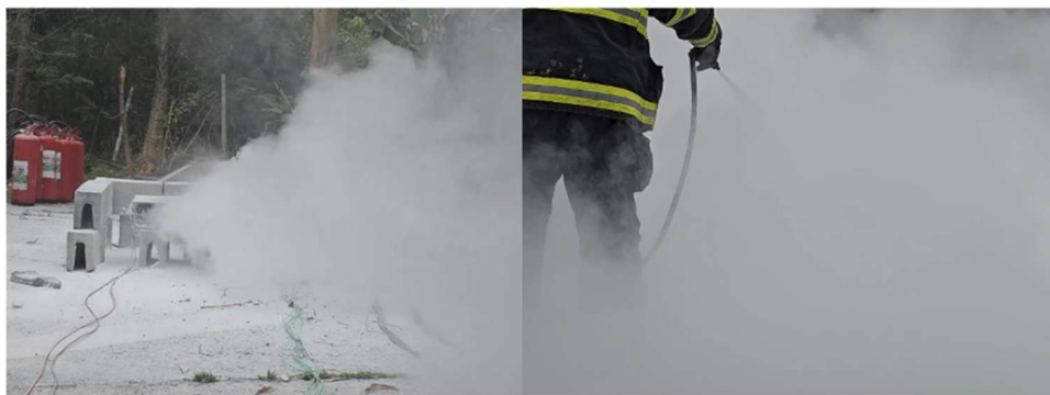
Figure 22 – Residual smoke emission after the third attempt (left) and the execution of a fourth mitigation intervention (right) (Battery C – Day 3).
