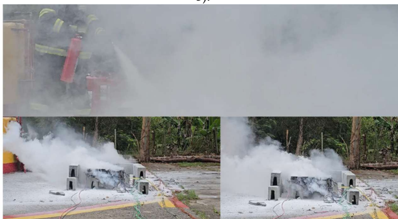
Figure 21 – Third intervention for smoke mitigation and subsequent re-intensification of emissions (Battery C – Day 3).
