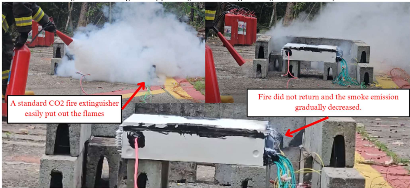
Figure 14 – Firefighter suppressing the fire using a extinguisher no Battery B.
