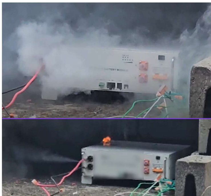
Figure 8 – Visual Record of Thermal Runaway and Deflagration (Battery A).
