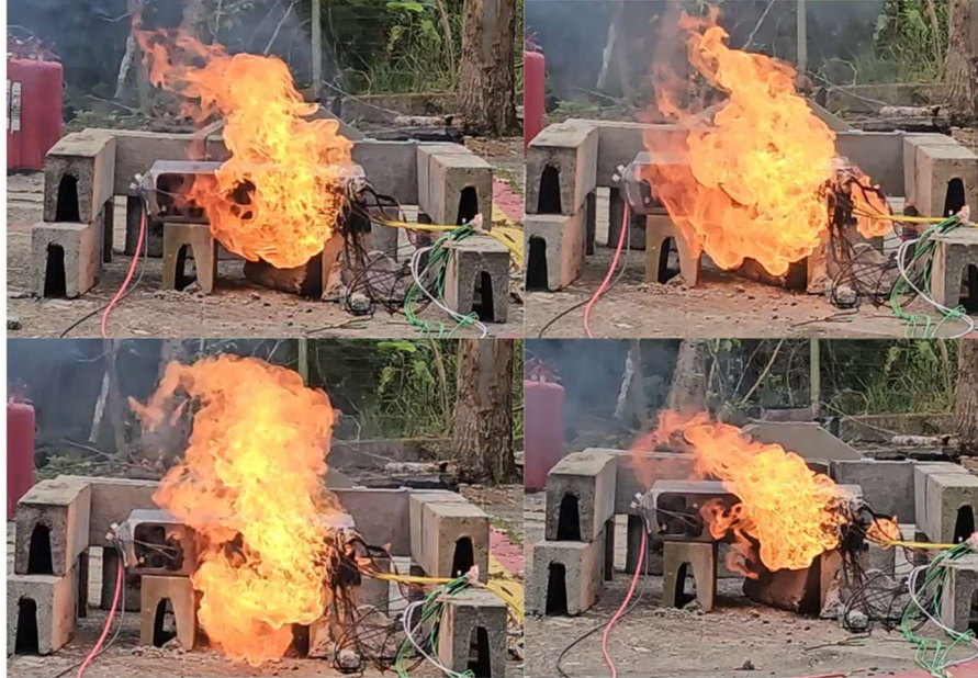
Figure 18 – Visual record of multiple explosions and jet fire (Battery C – Day 3)
