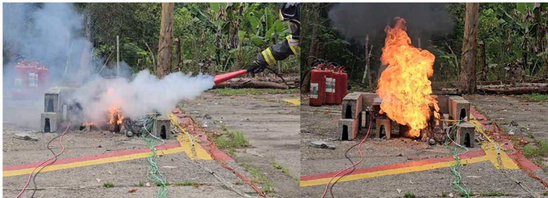
Figure 19 – Initial fire suppression attempt on Battery C and subsequent intensification of flames and explosions.
