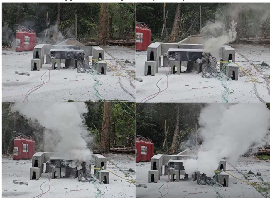
Figure 23 – Observation of temporary smoke reduction (top) followed by re-intensification (bottom) after the fourth suppression attempt (Battery C – Day 3).
