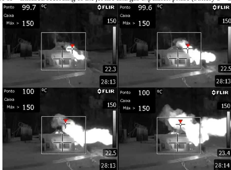
Figure 13 – Infrared recording of the jet fire and gas expulsion phase (Battery B – Day 3).
