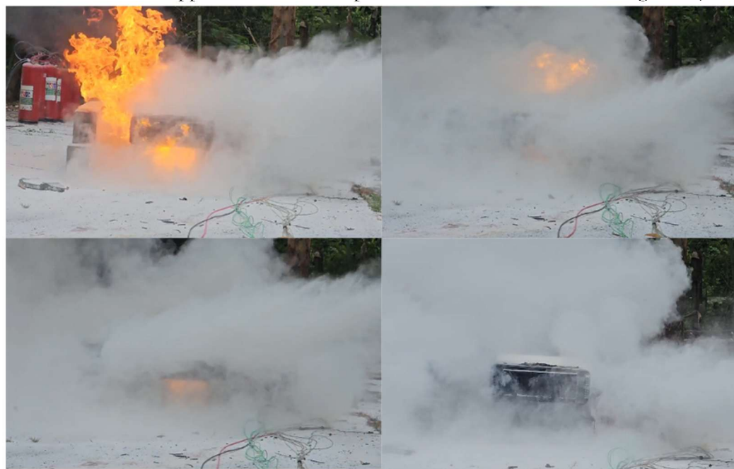
Figure 28 – Successful initial fire suppression and subsequent interventions for smoke mitigation (Battery D – Day 3).
